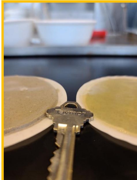
The filter cake on the left shows a CLEAR Slide Plus system with 10% solids and highlights the effectiveness of the system while managing drilled solids. The right shows 1% v/v lubricant embedded into the filter cake itself.
