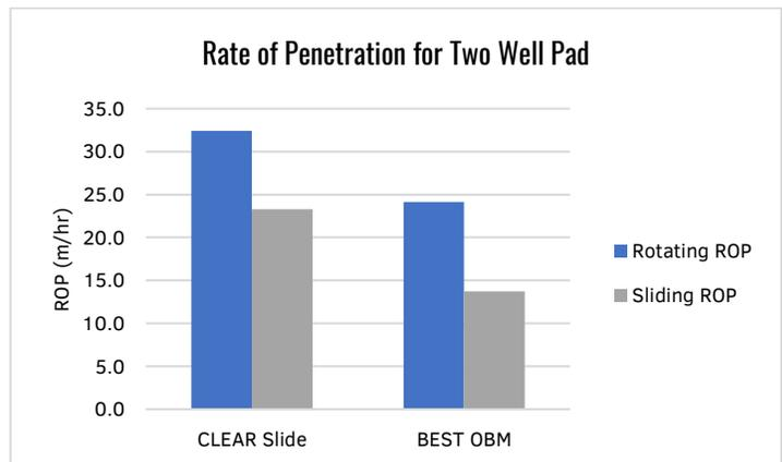
**Figure 2: Rate of Penetration Comparison for (12-12) pad**
