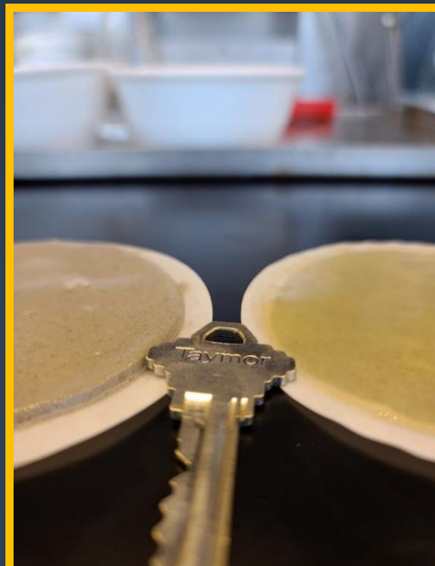
The filter cake on the left shows a CLEAR Slide Plus system with 10% solids and highlights the effectiveness of the system while managing drilled solids. On the right shows 1% v/v lubricant embedded into the filter cake itself.
